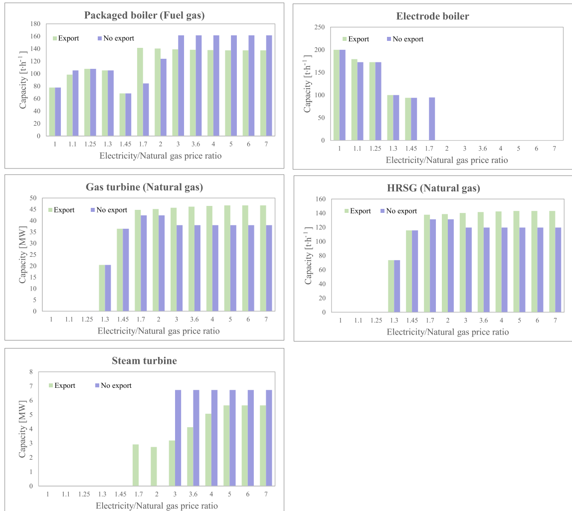
Figure 3-15 Results for the optimal process utility systems design based on the electricity/natural price and two scenarios characterized by hydrogen storage (HS) investment costs
